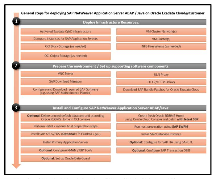
Figure 3: General Steps for Deploying NetWeaver Application Server ABAP/Java with Exadata Cloud@Customer X9M
