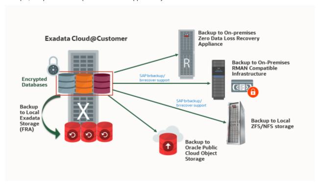
Figure 7: Oracle Database Backup Options with Exadata Cloud@Customer
