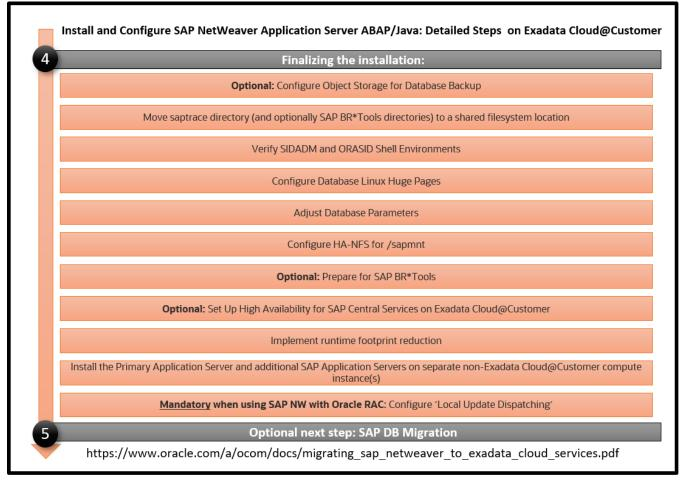
Figure 6: Steps to Finalize the Installation
