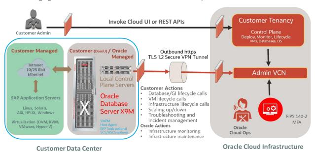
Figure 1: Architecture Overview of Exadata Cloud@Customer X9M with SAP NetWeaver
