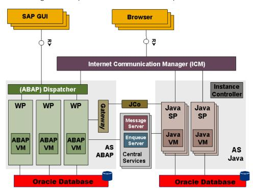
Figure 1: Components of the SAP NetWeaver® Application Server
